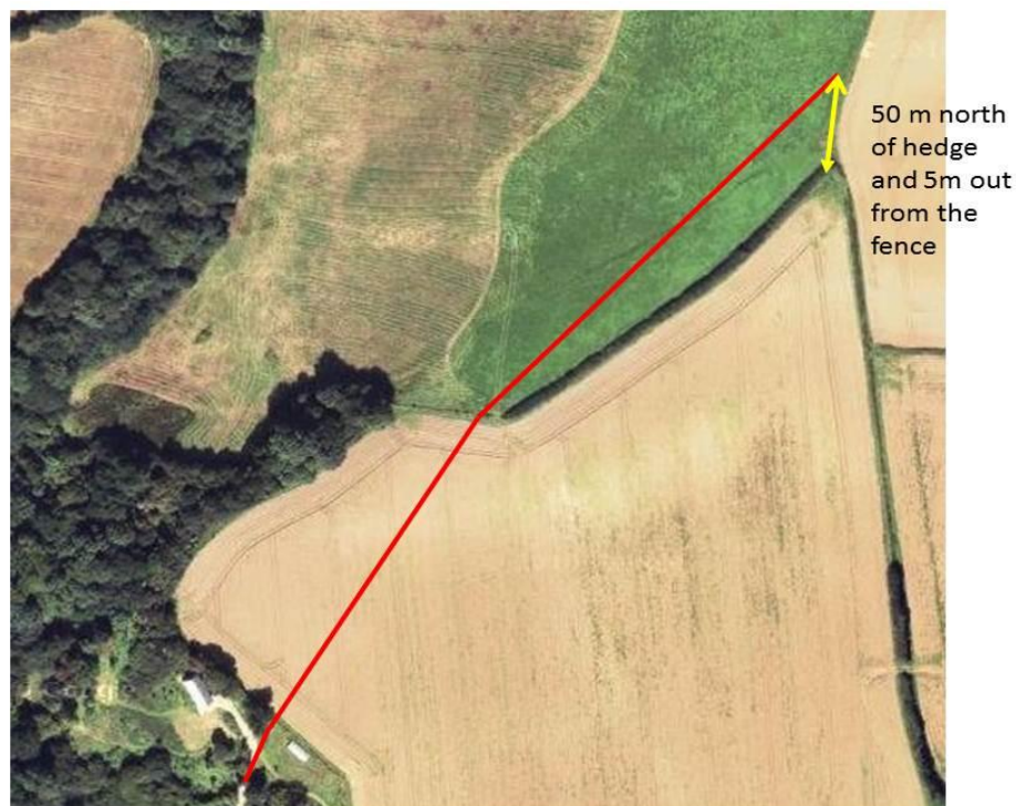
Figure 13. Cable run from turbine to 3 phase consumer board.
